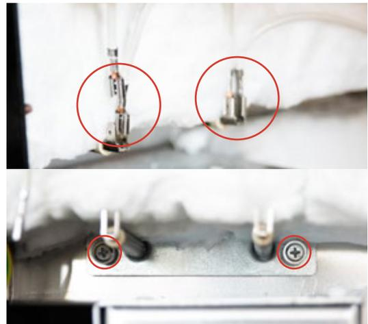
4. At this point disconnect the 2 electrical connection faston terminals and unscrew the 2 screws that attach the resistance to the oven structure. Unscrew the 2 fixing screws.
