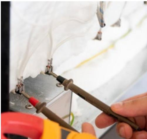
3. Identify the damaged resistor by checking the continuity of current between the resistors' poles using a tester. (This operation must be done by a specialized technician).
