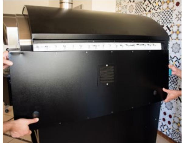
2. Once all the screws have been unscrewed, you can proceed to remove the side panel. It is advisable to have two people carry out the operation so as to avoid causing damage to the oven or the internal electrical circuit.
