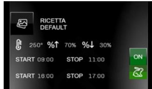
ON will start up pre-heating of the set recipe, according to machine configuration. The HARE will start up pre-heating in rapid heating mode if an analogue input has been configured.
