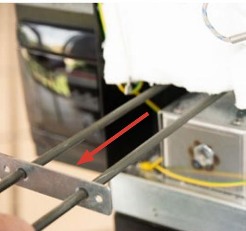
5. Remove and replace the resistor.
