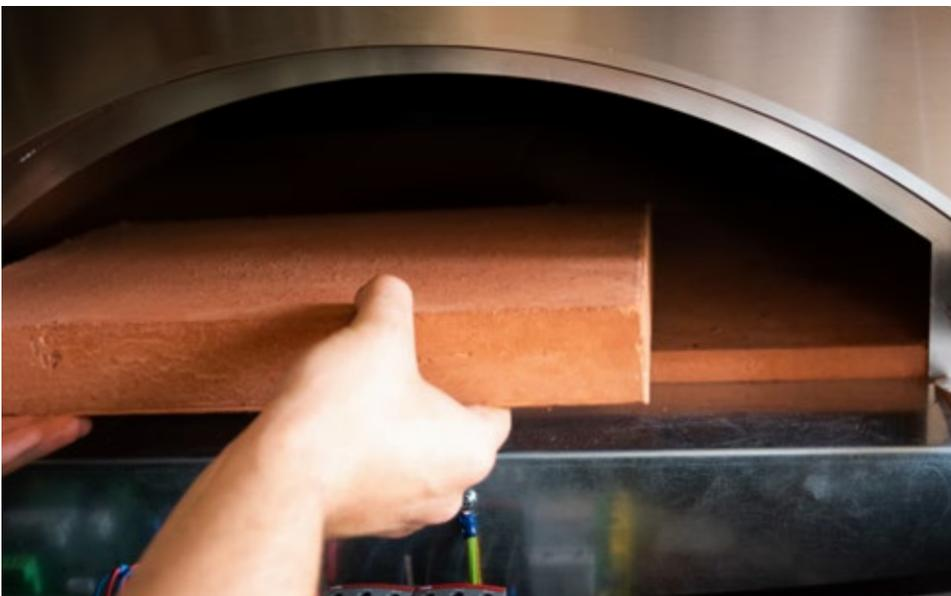
**3.** Replace the new tiles and reinstall the sill
