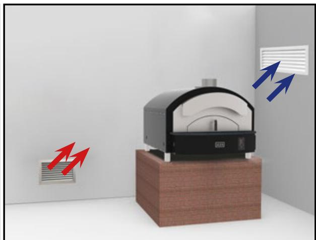
➔ **FORCED VENTILATION** -  $1,72 \text{ m}^3/\text{h} \times \text{kW}$
