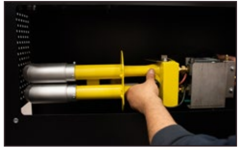
6 - - Remove the burner from the compartment
